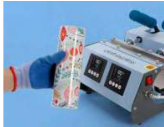
The two pressure handles also increase the pressure on the edge of the tumblers when you attach the long tumbler heater to this new mug press.
